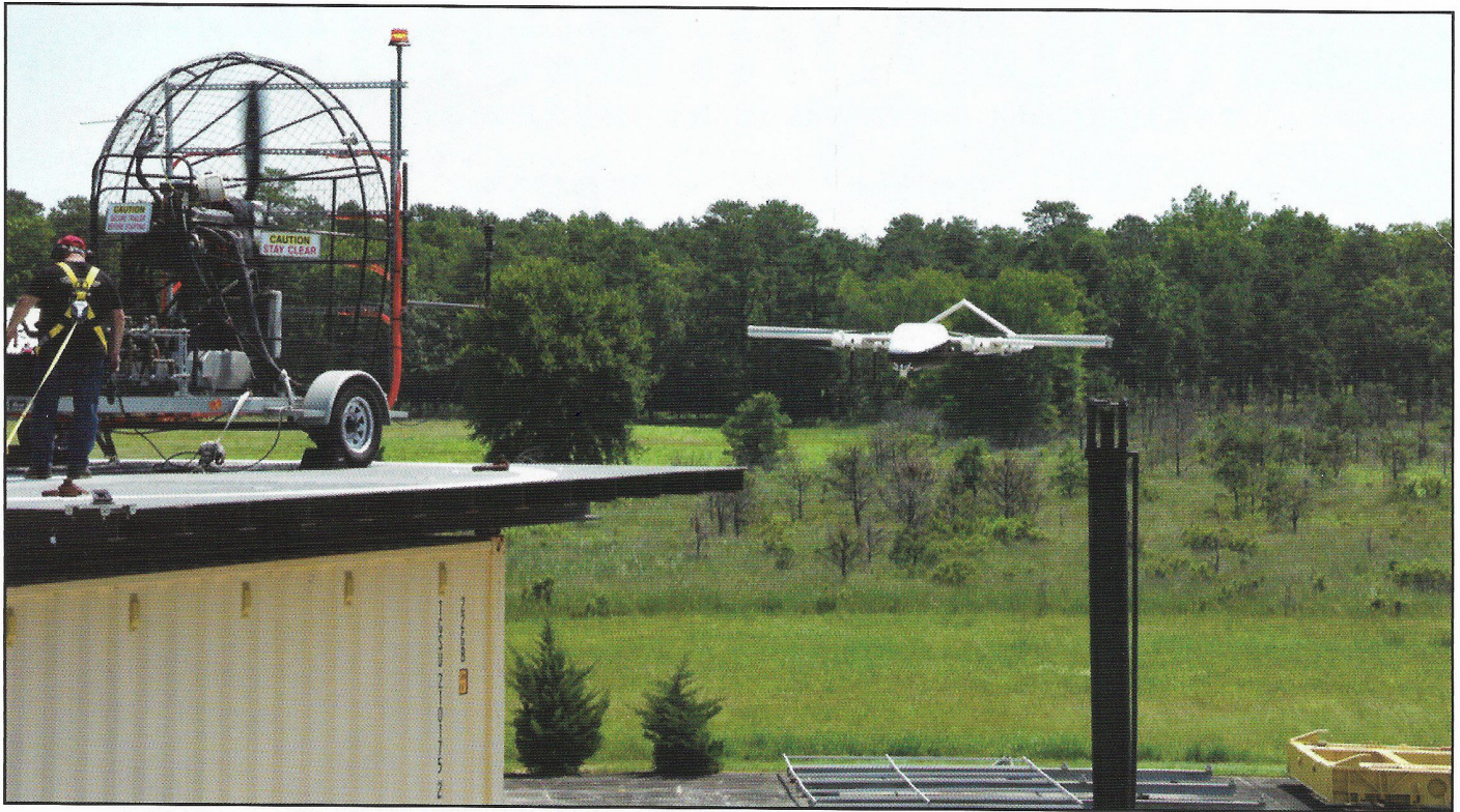
The Ship Motion Platform at Naval Air Warfare Center Aircraft Division Lakehurst can recreate sea conditions up to sea state 4 with wave heights of 4 to 8 feet. It can also be used to evaluate "Beyond-Visual Line of Sight" operations, flying a UAV to the limits of the Lakehurst airspace while being controlled from the SMP test site. (U.S. Navy photo)
